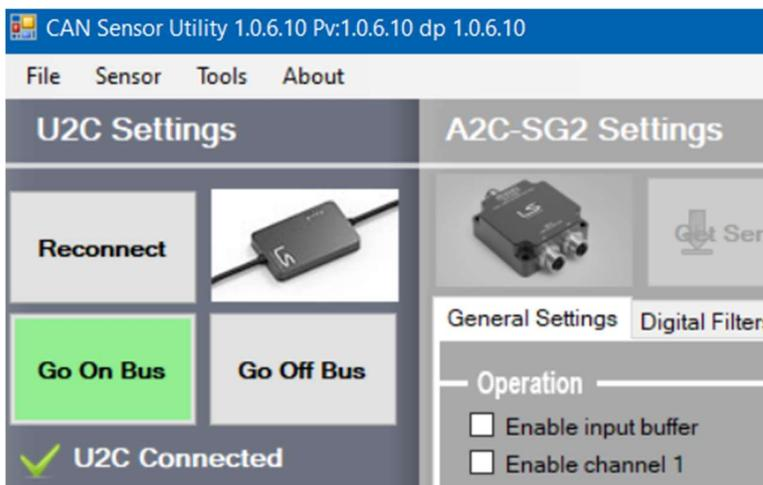
Figure 3 Go On Bus to enable communication
