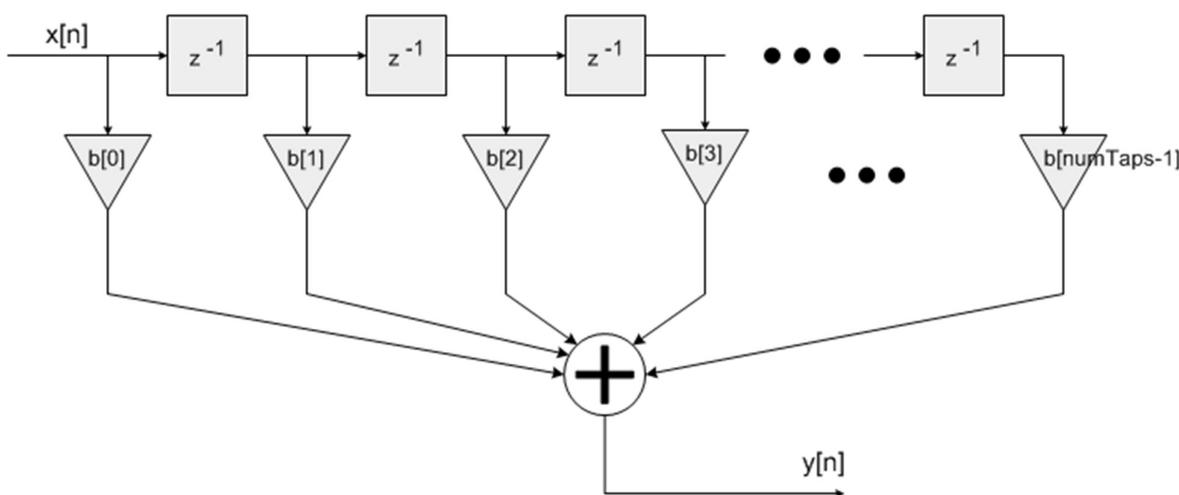
The coefficients points to a coefficient array of size numTaps. Coefficients are stored in **time reversed order**.
